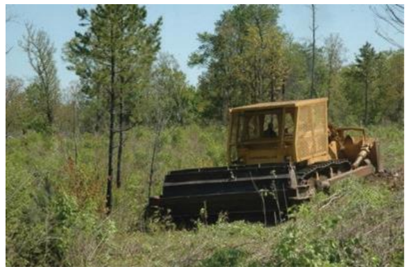
Drum-chopping can be used to set-back succession where shrubs and trees have gotten too large to allow disking or mowing and where the application of prescribed fire is not an option.
